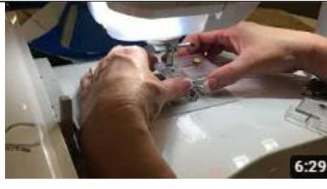
[Attaching Feet to Higher End Sewing Machines](#)
